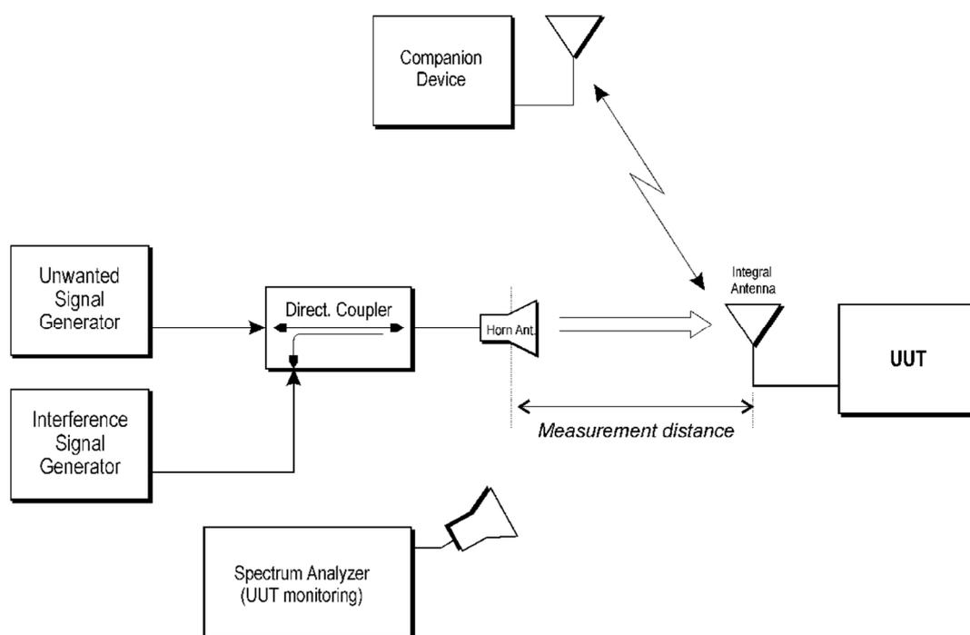
**Figure C.2: Measurement Set-up**
